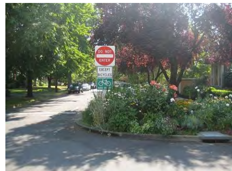
Traffic calming on some streets in Central Eugene results in a more comfortable bicycling experience.
